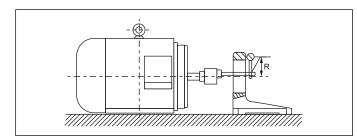
The mounting speed of the pump on the bracket is checked against the verticality of the output shaft of the prime mover.
