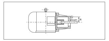
The verticality error is  $\emptyset 0.05$  (R is the diameter on the distribution hole of the pump mounting screw hole) pump shaft mounting hole check the vertical mounting angle of the flange
