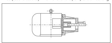
Coaxial error is  $\emptyset 0.05$  pump shaft mounting hole on the flange mounting hole coaxial check
