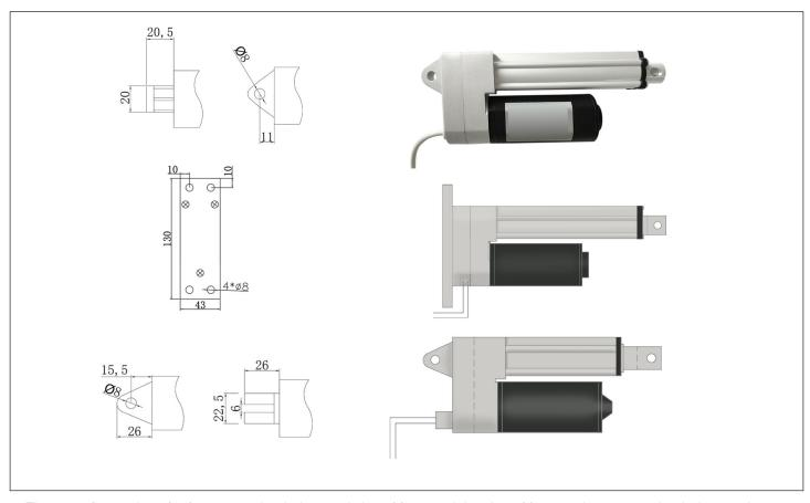
There are five options for front mounting holes, and size of front and the size of front and rear mounting holes can be cust-omized as required.
