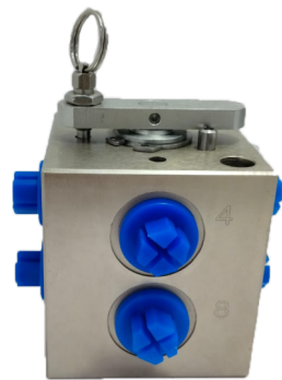
2 Position 8 way switching valve Flow rate: 20 L/min Rated Pressure: 100 Bar
